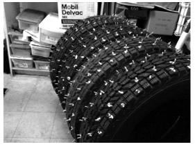
screws were inserted into and through the tread each tire. The protruding points were ground down to a uniform length of 3/16". The resulting screwed tires
