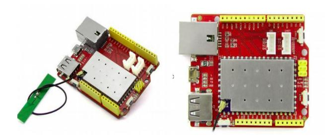
This device is based on the Atheros AR9331, @400MHz chipset.
