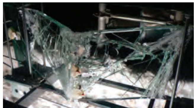
Test with temperature load: Fracture pattern
