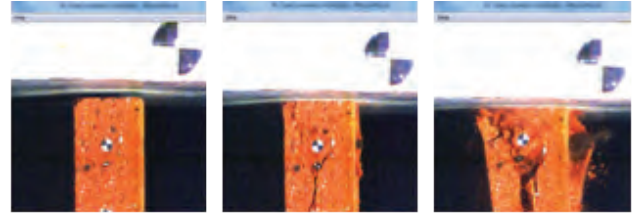
Typical high-speed test sequence for clay brick under compression
