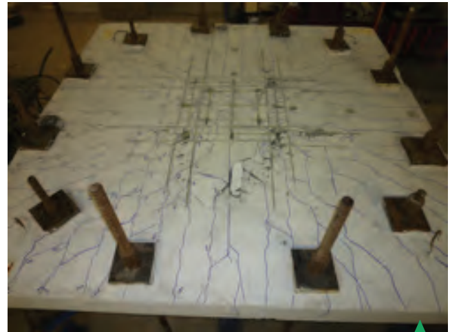
RC slab strengthened to flexural and punching according to the new technique and CFRP laminates
