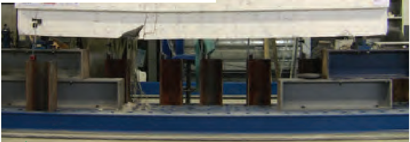
RC beam strengthened in flexure and shear according to the new technique and CFRP laminates
