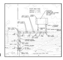
The project entails a raised boardwalk ramp structure, gangway, and floating dock with a platform and rail allowing for wheelchair transfer into a kayak. A
