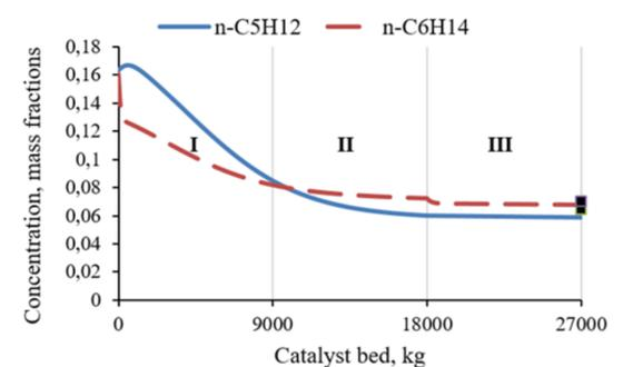
Fig. 2. N-pentane and n-hexane concentrations profile. Vertical lines correspond to the reactor section zones I-III
