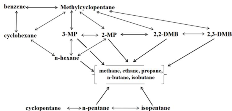
Fig. 1. Transformations of the catalytic isomerization of the pentane-hexane fraction (2-MP – 2-methyl pentane; 3-MP – 3-methyl pentane; 2,2-DMB – 2,2-dimethyl butane; 2,3-DMB – 2,3-dimethyl butane)
