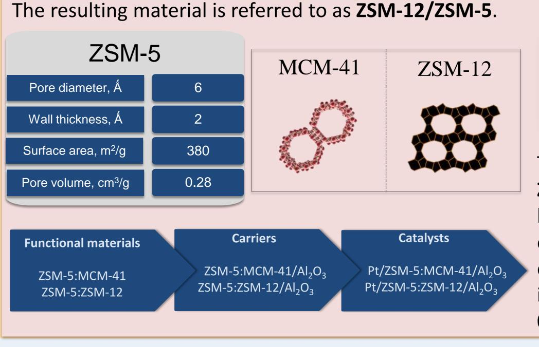
The resulting composites **ZSM-5:ZSM-12**, **ZSM-5:MCM-41** were mixed with bohemite in 60:40 % wt. ratio and extruded, then Pt was deposited over the extrudates by incipient wetness impregnation method in the amount of 0.5 % wt.
