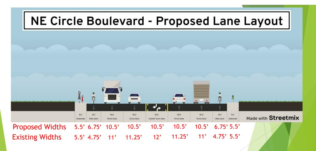
Re-apportioned vehicle lane widths to create 2-ft buffers for both bike lanes.
