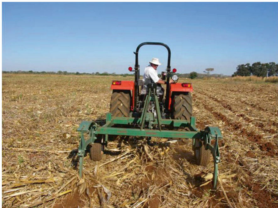
Fig. 2 Conservation agriculture with ripping and retention of crop residues as mulching (Photo by CFU Zambia)
