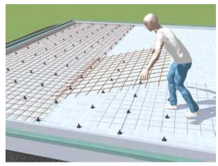
The U-Sinus Ties should be placed at the same level as the reinforcement mesh, 50mm from top of RC Slab. Pre-drill holes in inner flange of the element c/c 900mm unless otherwise is specified on your work drawing. Position the ties as shown on the picture.
