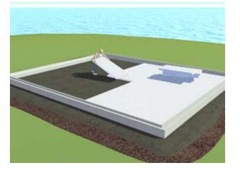
**5** • All corner elements are cut to the correct angle and fixed with Fixkil, a toothed metal plate as shown on the picture. Allways check the angle.
