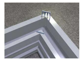
Roll out the radon barrier on tp of the first insulation layer. Over lap with minimum 300mm. Fit sleeves on services comming through the insulation.
