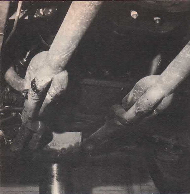
The "bundle of snakes" type headers proved to be the most difficult part of this special engine package. Each header pipe is the same length and empties into a Gran Prix type collector.
