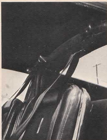
Foam rubber is molded around the sturdy roll bar (Shelby standard) to keep heads from being cracked on entry to the rear seat. Retractable shoulder harnesses are also standard equipment.
