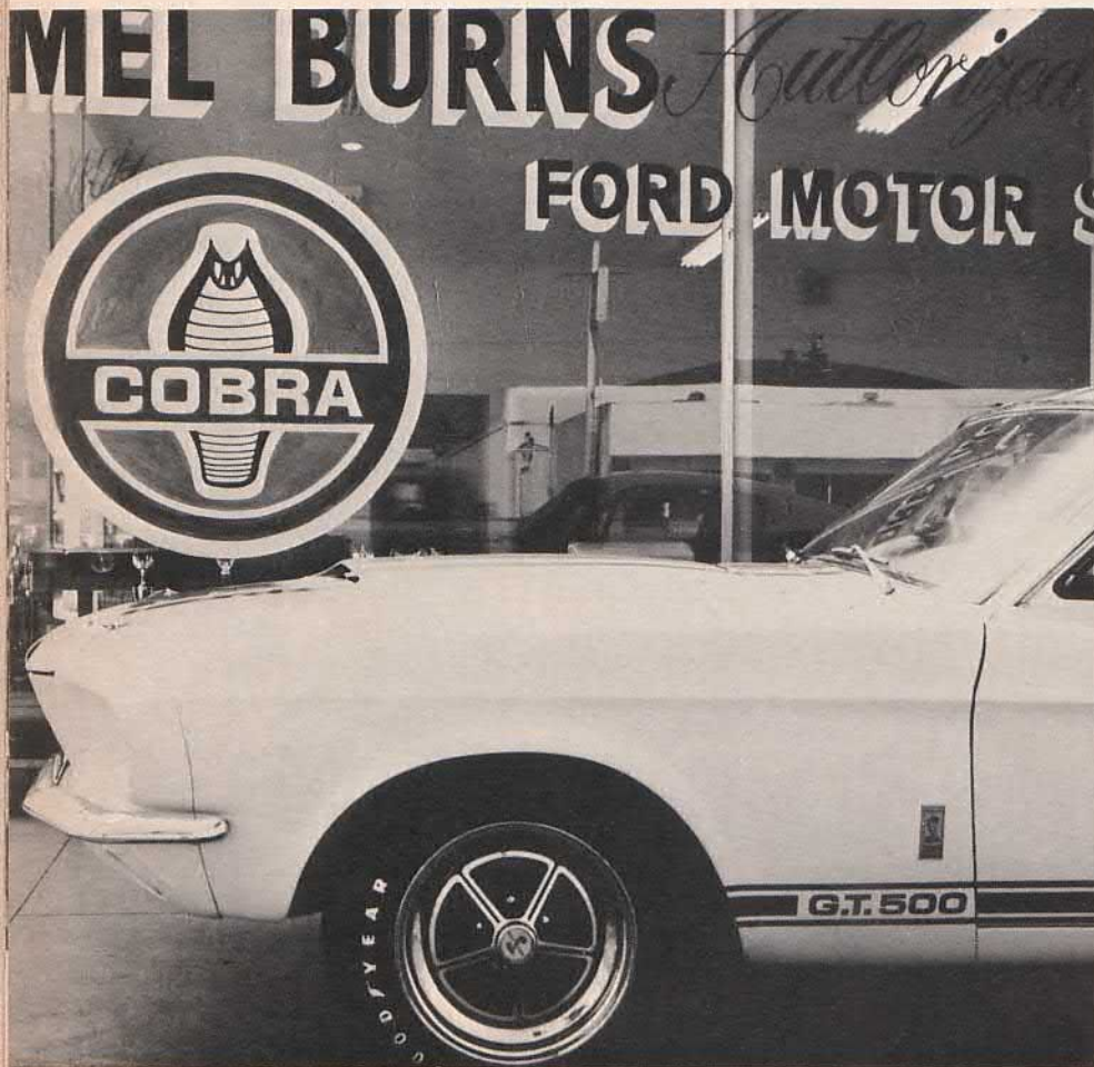
Fiberglass hood and front grille housing panels extend the GT's overall length by three inches, giving it an even sportier appearance than the standard Stang.
