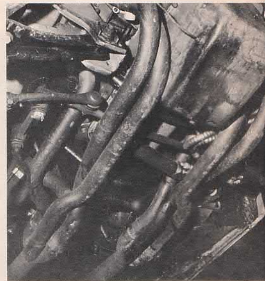
Large 8 qt. oil pan supplies plenty of oil to the engine's lubrication system. Special 4-into-1 headers were fashioned by the wizards from the Cobra works.
