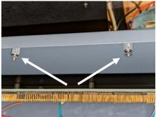
5) PTC fuses at W2 and W3 must be carefully positioned when soldered into place to avoid interference with a board installed at new expansion slot P16
