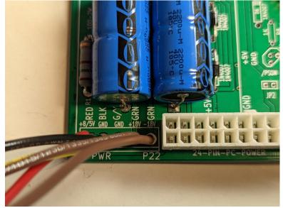
If you elect to use terminal block P22, consider the clearance available between the 2200uf filter
