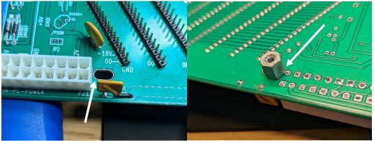
Heath used 3/8" hex standoffs for the backplane. You can see from the second photo that there is a possibility for contact with the pins of P21 if the board is pulled all the way forward in the mounting slots when mounting. This is only an issue if you are planning to use P21 and an ATX-style power supply attachment to the backplane. Possible solutions:
