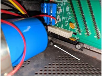
The backplane fits snug against the bottom of the H8 case. Interference between the foot mounting screw and P22 forced the board about 1/16" out of alignment. Possible solutions:
