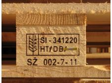
This pallet was made in Slovenia (SI) by the supplier 341220, the pallet was Heat Treated (HT) and debarked (DB). The Pallet was made in July 2011. This pallet is safe to use.
