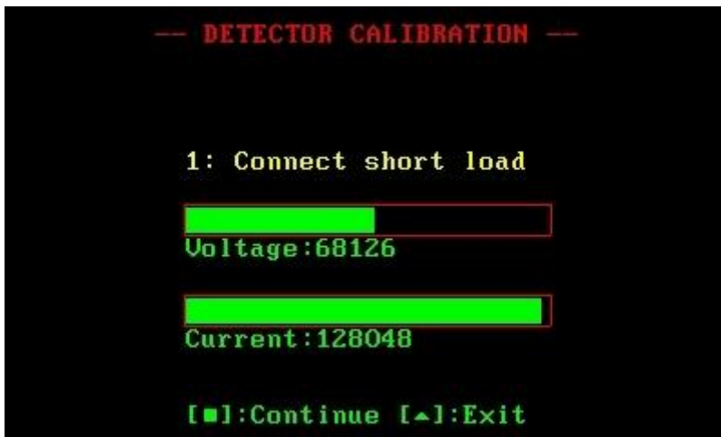
Figure 3, Short load condition
