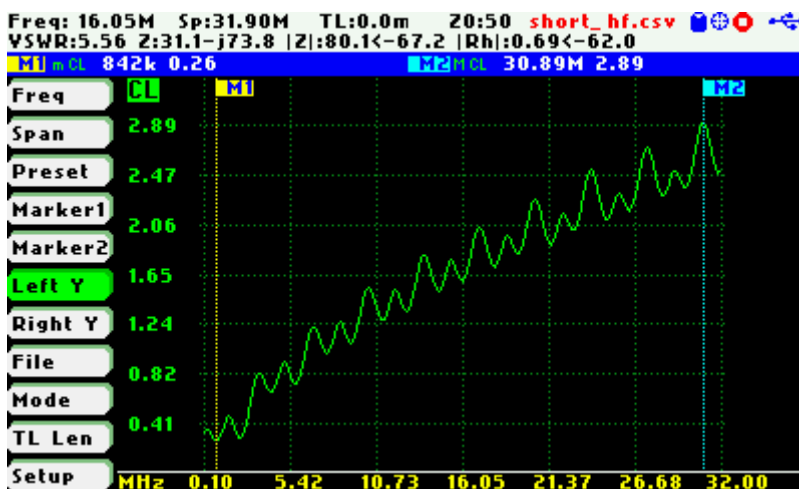
Figure 2, typical insertion loss display in SARK-110 screen
