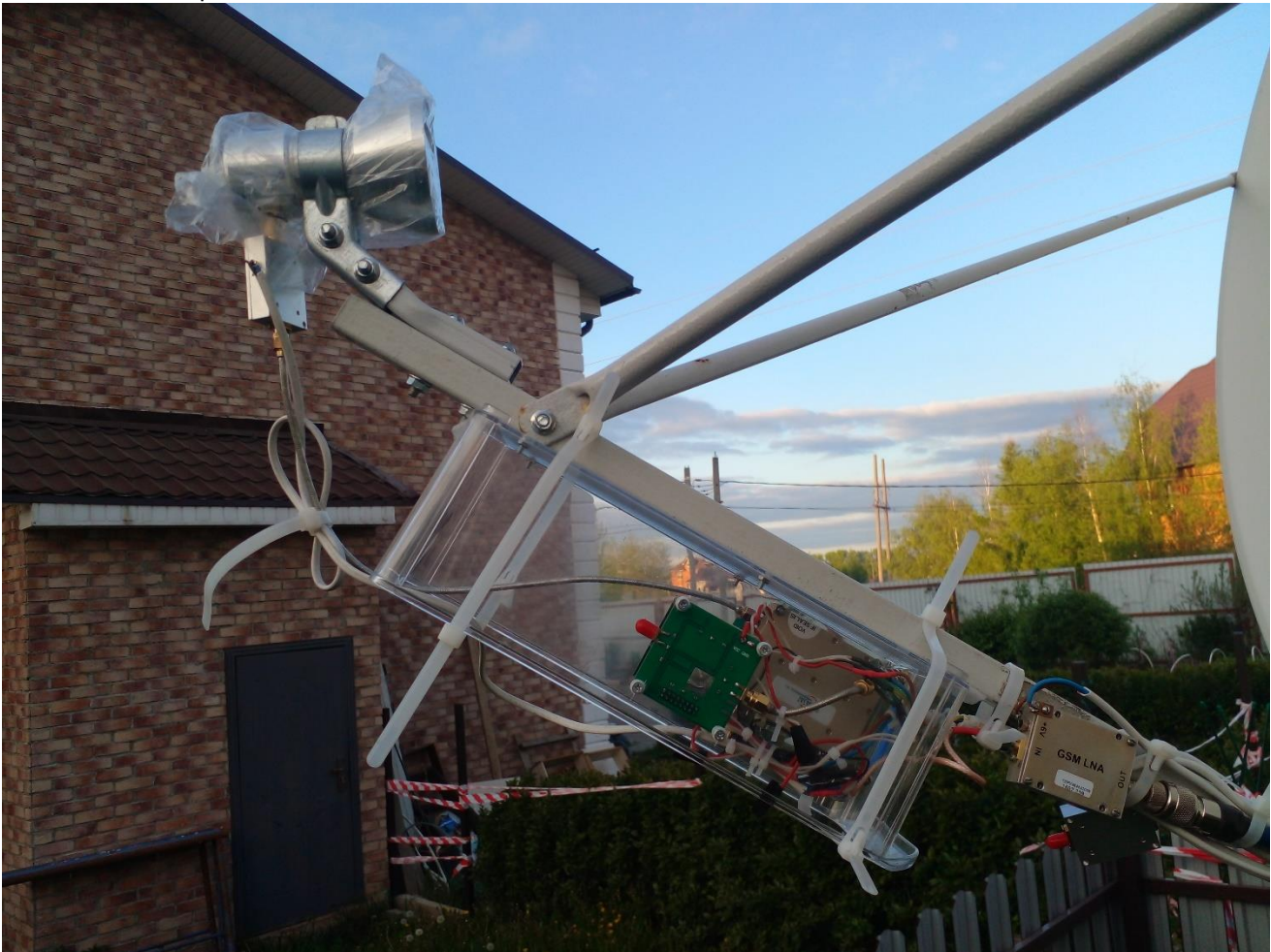
Receiver outdoor part with the module Terraset 6.4-7.1 GHz:
