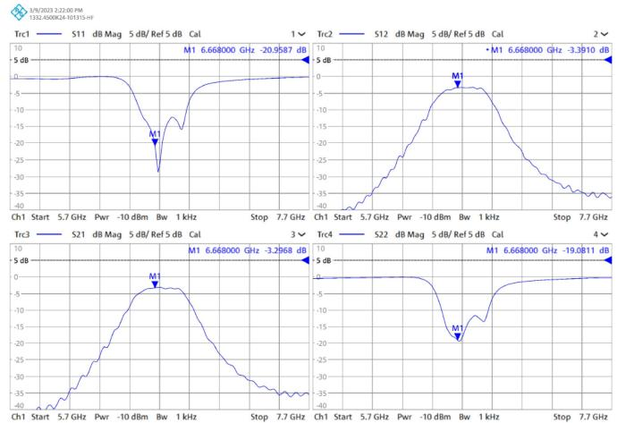
Transfer characteristic slopes are not too steep, but the stopband attenuation is acceptable for the receiver.
