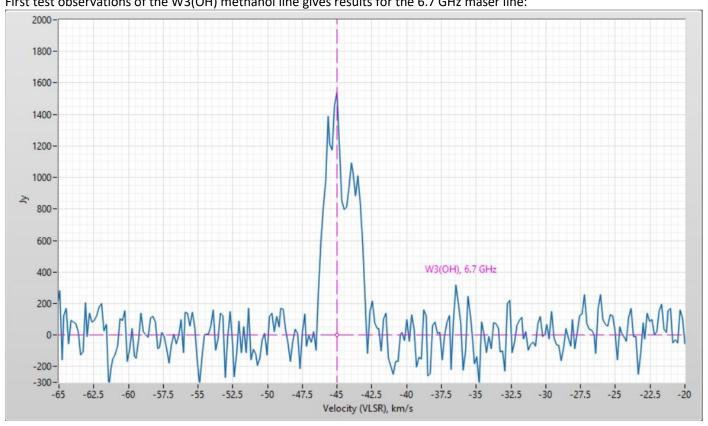
Integration time was about 40 min, receiver resolution – about 5 kHz (0.2 km/s in the VLSR scale), the dish position was controlled by automatic tracking of the source. Expected line width and peak velocity are reproduced well, but received peak level is somewhat lower than expected >3000 Jy. There was a real snowfall during measurements; the atmospheric absorption was taken 1 dB, but higher absorption values were also probable.
