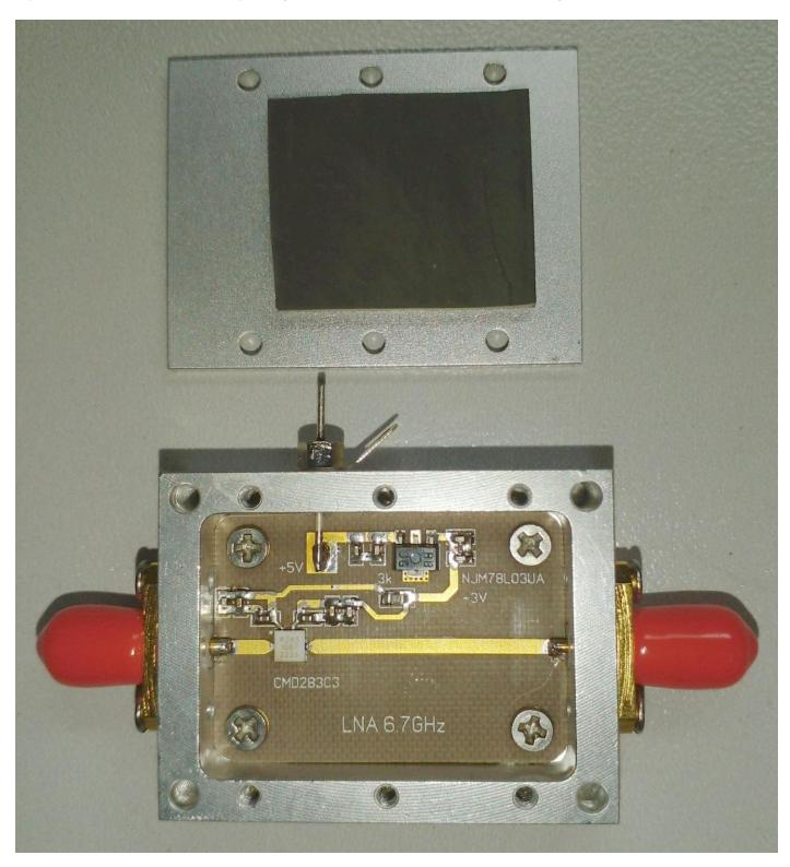
Noise Figure and insertion Gain are at the plot next (measured by R&S FSV with noise head NC346A Precision). A better Noise Figure was expected at 6.7 GHz according the plots in the CMD283C3 datasheet (about 0.8-0.9 dB), but just 1.16 dB was received. Nevertheless, it is better than in available LNA from Mini-Circuts
