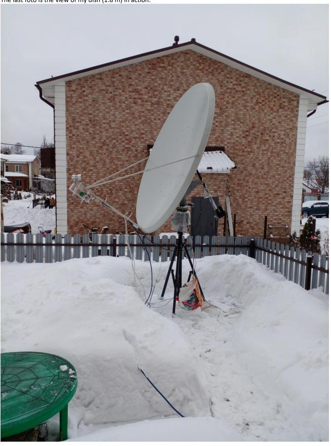
Dish telescope characteristics: Antenna Sensitivity (Forward Gain) -0.63 mK/Jy,  $T_{sys}$  was 200 K or higher this day (including the atmospheric thermal noise).
