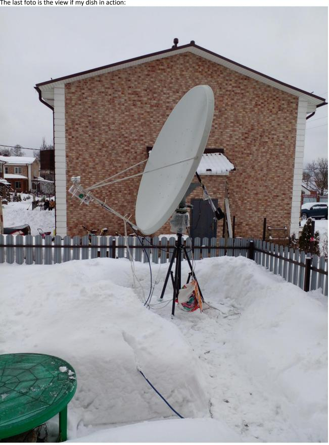
Dish telescope characteristics: Antenna Sensitivity (Forward Gain) -0.63 mK/Jy,  $T_{sys}$  was this day 200 K or higher (including the atmospheric thermal noise).
