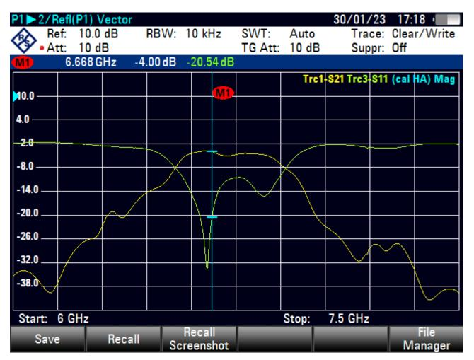
Transfer characteristic slopes are not too steep, but the stopband attenuation is acceptable for the receiver.
