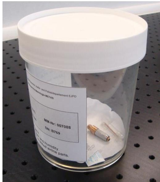
In order to minimise oxidation each un-plated BeCu Air Line is stored in special storage box which is filled with Argon gas and a desiccant bag.
