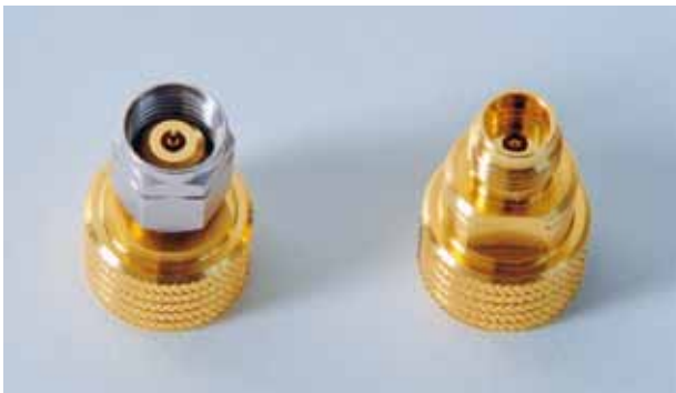
1 The metrology grade 1.85 mm connector (male part on the left and female part with slotted inner conductor on the right) is applicable for frequencies up to 67 GHz. The diameters of outer and inner conductor are only 1.85 mm and 0.8036 mm, respectively. The small dimensions make this connector particularly delicate to handle.
