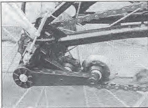
H. Here's the part that gives me the willies—the weird and unfamiliar chain tensioner and internal gearshift mechanism.
