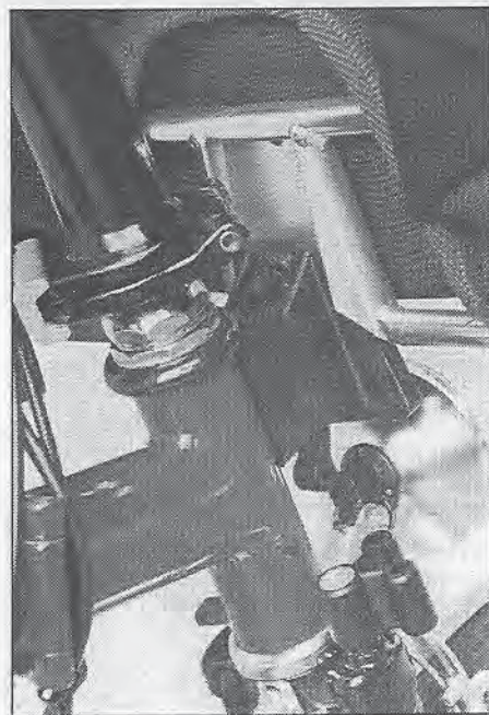
J. Here's the stout metal rack of the front pannier sliding solidly over the block. There's a trigger release below it, cleverly hidden from criminals who would have what is rightfully yours, yet convenient enough for a 2-second quick release.
