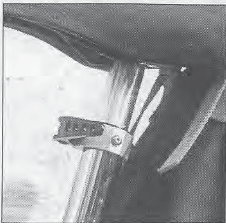
P. An optional telescopic seat post extension accommodates guys with really long legs. You can also get a longer standard seat post. Oh heck—if you really want to know more, get a brochure from Channell Wassoon.
