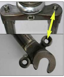
There's a lot going on with these three pix, so please pay attn. The tapped fork crown and top eyelet on the front dropout allow creative rack mounting that wouldn't be possible without them. Tubus rear racks on the front, for example; or the R14 Top rack (and another we have in the works) on the front.
