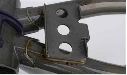
It's a chainstay-bridge! It's a kickstand plate! It's a double-duty hunk of metal. A Pletscher kickstand bolts right on, adding just 7.2 ounces to a bike that doesn't count ounces.
