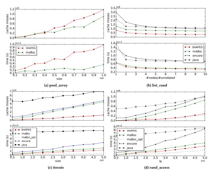
**Figure 6.** Comparison of pools against arrays and pointer-based data structures. Smaller is better in all the plots. Cache misses and time plots share the same x-axis.
