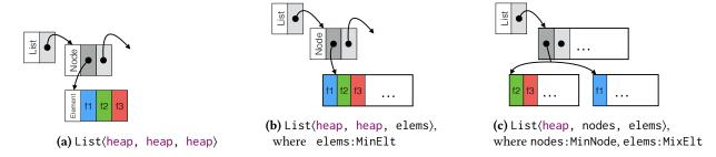
**Figure 5.** Three different layouts for the same data structure.
