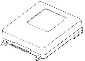
The RTZW-02 provides two-way communication as part of a Z-Wave® network. When it receives commands from Controller device, it sends back confirmation that the command was received and implemented. Each module in a Z-Wave® network communicates with every other module, acting as a "repeater" and routing your commands to their destination
