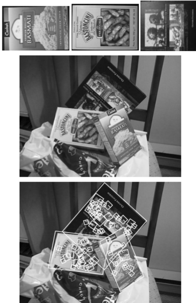
Figure 1: SIFT algorithm finds keypoints in an image, i.e. localized features that are particularly useful for identifying the objects in an image. The top row shows images that are matched against the image in the middle row. The bottom-row image shows some of the keypoints used to perform the matching (i.e. these keypoints demonstrate the same features in the top-row images and their transformed middle-row counterparts). SIFT keypoints are identified via a staged filtering approach. The first stage identifies key locations in scale space by looking for locations that are maxima or minima of a difference-of-Gaussian function. Each point is used to generate a feature vector that describes the local image region sampled relative to its scale-space co-ordinate frame. The features achieve partial invariance to local variations, such as affine or 3D projections, by blurring image gradient locations
