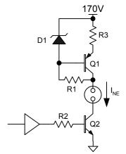
High side constant current linear drive. Q1 dissipates all of the waste heat, voltage on R3 is usually very low compared to the voltage across Q1. Multi segment displays can share Q1 and the segment drives can be either NPN or MOSFET saturated switches. I<sub>R1</sub> needs to be about (I<sub>R3</sub> / 100) to satisfy Q1 h<sub>FF</sub>.
