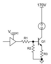
Low side constant current linear drive. Q1 dissipates all of the waste heat, voltage on R3 is usually very low compared to the voltage across Q1. Requires a current sink for each segment. This will not work with MOSFETs.  $I_{\rm R1}$  needs to be about ( $I_{\rm R3}$ / 100) to satisfy Q1  $I_{\rm Rc}$
