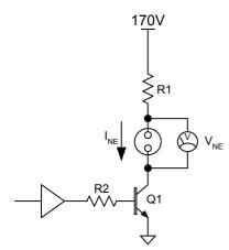
Simple saturated NPN drive. R1 dissipates most of the waste heat, the voltage across Q1 is usually nearly zero. One limiting resistor shared by all digits, but current varies with changes in 170 rail. I<sub>R1</sub> needs to be much greater than (I<sub>D1</sub> / 100) to satisfy Q1 h<sub>EE</sub>.
