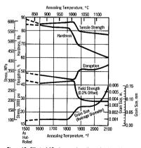
Figure 18. Effect of 15-min anneal on the grain size and roomtemperature mechanical properties of an INCOLOY alloy 800 hotrolled round 17/32 in. (31 mm) in diameter.
