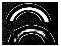
Figure 21. Hot-bent Nickel 200 tubing. The lower specimen was bent using sulfur-contaminated filler sand. The upper specimen was bent using sulfur-free filler sand.
