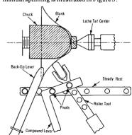
Figure 5. Typical equipment for manual spinning.
