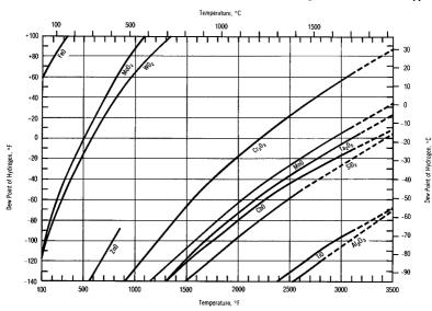
Figure 15. Metal/metal oxide equilibria in hydrogen atmospheres.2
