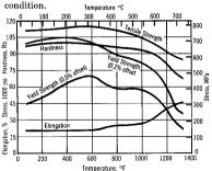
Figure 17. Effect of heating temperature (3 h at temperature) on the room temperature mechanical properties of a MONEL alloy 400 cold-drawn rod
