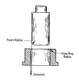
Figure 2. Critical areas in designing deep-drawing equipment.
