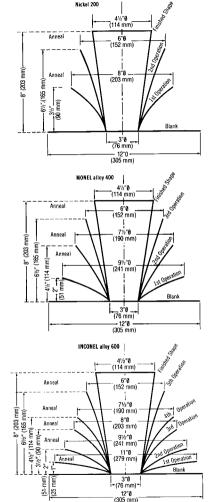
Figure 7. Sequence of operations for spinning deep cups from 0.037 in. (0.94mm) thick blanks of Nickel 200, MONEL alloy 400 and INCONEL alloy 600.
