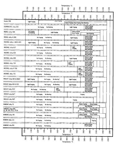
Figure 20. Temperature ranges for hot forming.
