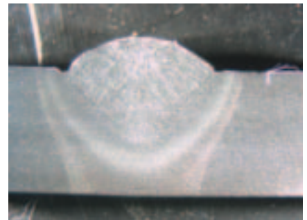
Fig. 3 — Undercut generally occurs when the amount of wire deposited is not great enough to fill the gaps in the material caused by the voltage. This can be avoided by reducing travel speed, increasing current, or decreasing voltage.
