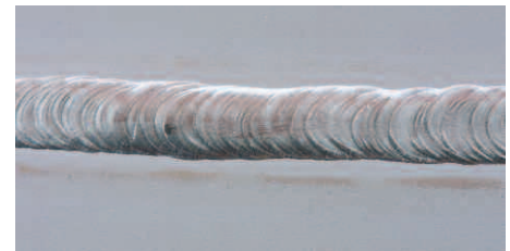
TIG seam, root side, with root protection
