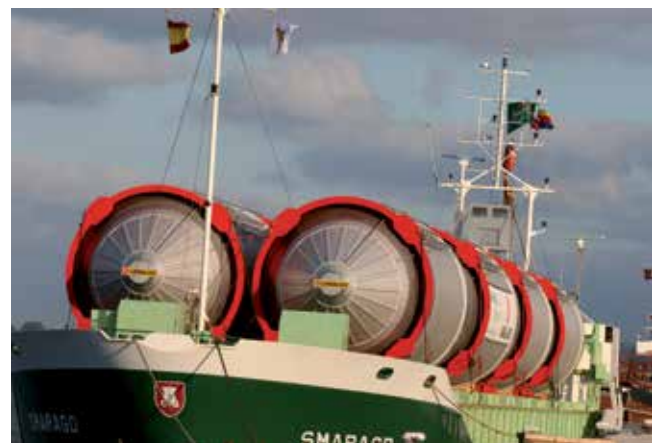
Stainless steel beer tanks ready for shipping after complete cleaning using Avesta products. Photo courtesy of Landaluce.
