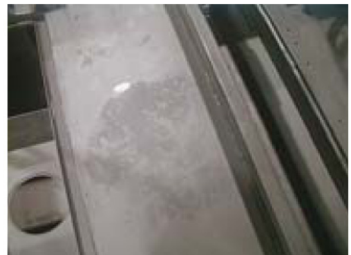
Patchy, uneven pickled surfaces can result if surfaces are not clean before the acid treatment.
