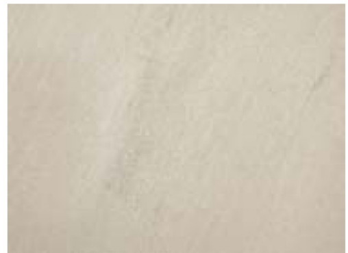
A matt grey is left on annealed mill products following descaling and pickling. Mechanical scale loosening roughens the surface.
