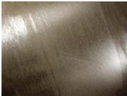
Stainless steel surfaces form a grey/black scale during hot rolling or forming. This tenacious oxide scale is removed in the steelmill by descaling.
