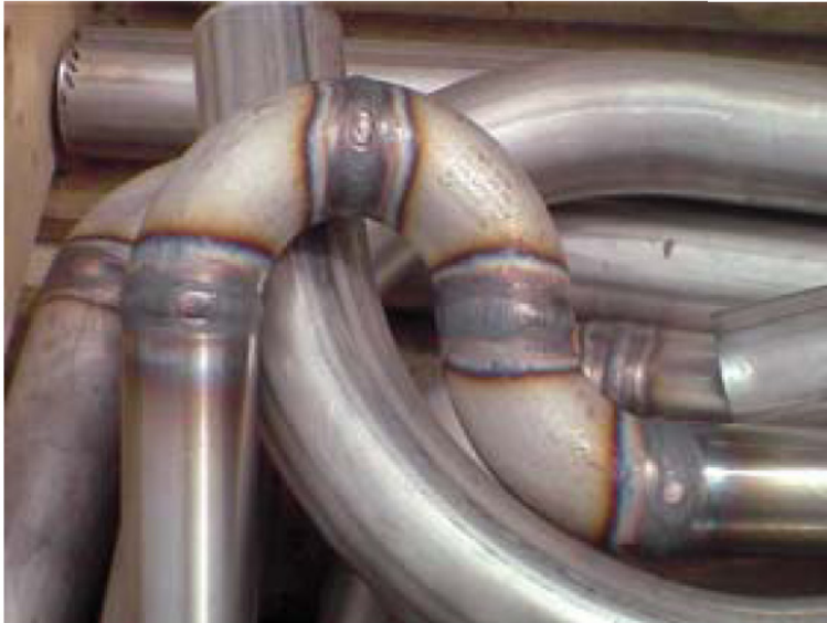
Light scaling left on weld caps and heat tint on the surrounding parent tube surfaces can usually be removed by acid pickling.
