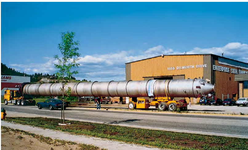
2205 oxygen delignification reactor, Enterprise Steel Fab, Kalowna, Prince George, British Columbia, Canada (Source: Outokumpu)
