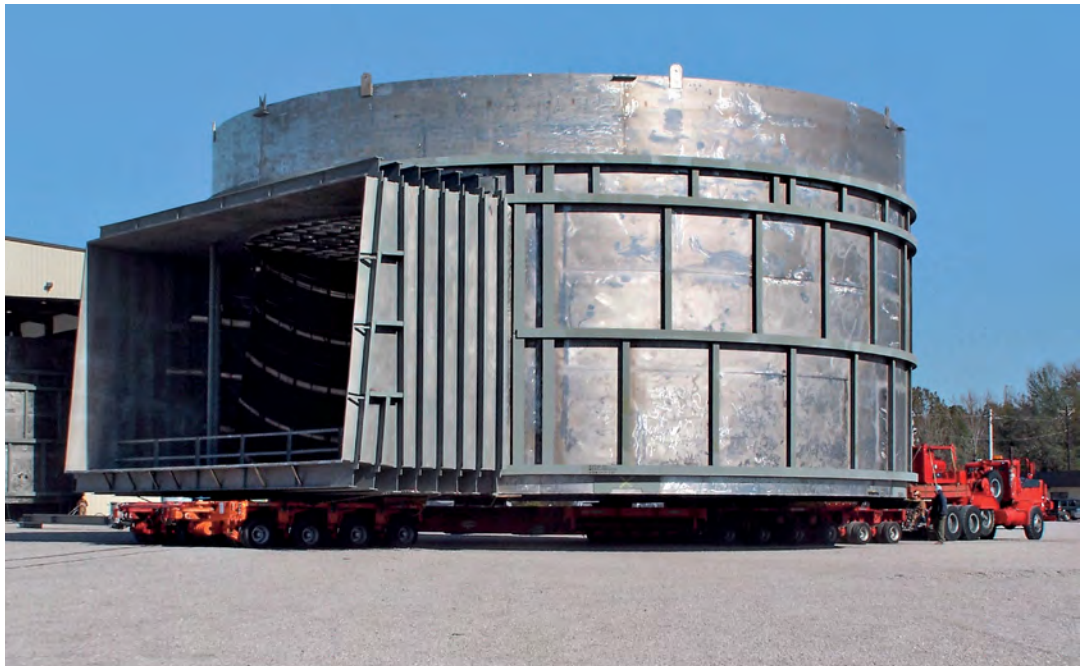
Flue gas desulfurization unit fabricated using 2205 stainless steel (Source: ArcelorMittal)
