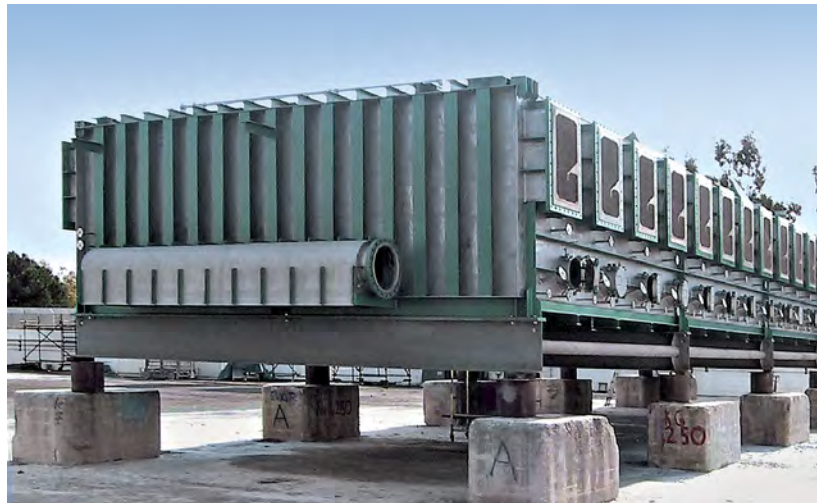
Multi stage flash seawater desalination unit constructed of S32101 and S32205 duplex stainless steels (Source: Outokumpu)
