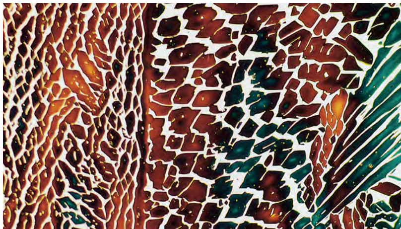
Metallographic structure of 2205 duplex weld metal, 500x (Source: Lincoln Smitweld bv)
