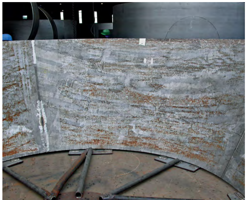
Embedded iron in roll formed duplex stainless steel plate fabrication (Source: Gary Carinci, TMR Stainless)
