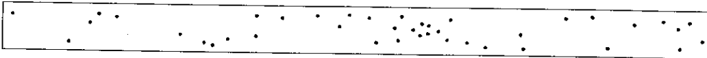
Typical Quantity and Size Permitted in 6 in. (150 mm) Length of Weld \frac{1}{8} in. (3 mm) to \frac{1}{4} in. (6 mm) Thickness
