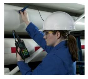
**Application:** Accurately measuring remaining wall thickness of metal pipes, tanks, beams, ship hulls, and other structures through paint and similar coatings.
