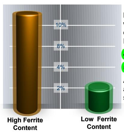
In Benefits- a ferrite level of at least **3FN** will eliminate fissuring (starting points of cracks) in weld metal deposited by E308,E308L,E316,E316L
