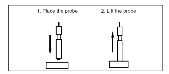
The probe has to be lifted at least 50 mm (2") from the measuring object between readings.
