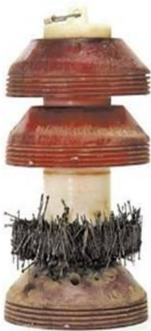
TDW 8" 3C-MAG Magnetic Cleaning Pig after 177 mile (285 km) run
