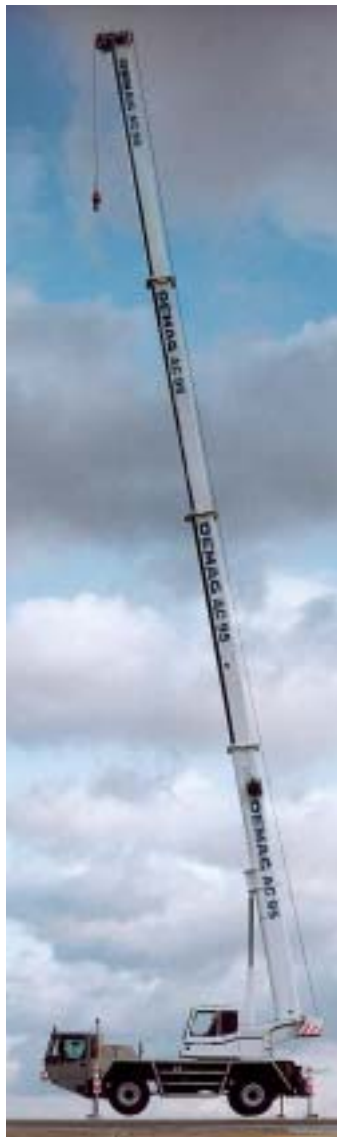
Figure 1: Crane booms of this length would not be conceivable without modern steels such as DILLIMAX (Illustration used with the kind permission of Demag Mobile Cranes GmbH, Zweibrücken, Germany)
