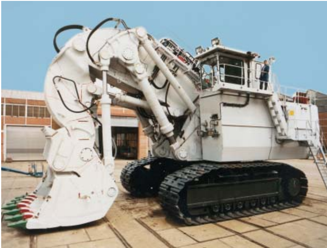
Figure 4: O&K hydraulic excavator RH 400: Load bearing structural components made of DILLIMAX 690 T (Illustration with the kind permission of the Orenstein & Koppel AG, Dortmund, Germany)
