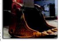
on 14% Mn steels, hard or unidentified steels. Very thick build-ups possible without cracking. Specially developed for mining industry.
