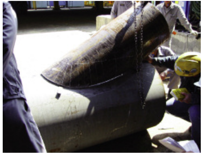
Fig. 5 — The author demonstrating the measurement of the brace intersection angle at the heel of the joint. The fitters were being trained to do this as part of verifying the proper location of the brace member prior to tacking.
