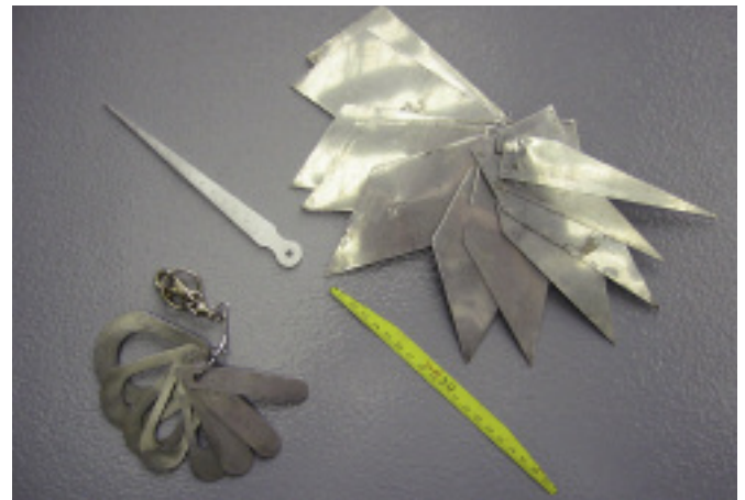
Fig. 2 — Typical TYK inspection/measurement tools, including clockwise from top left: root opening gauge, dihedral angle/groove angle gauges, W dimension rule, improved surface profile radius gauges. Note that the ends of the rule have a tapered cut at a dimension equal to the required W dimension that will allow the rule to be inserted into the root of the joint.
