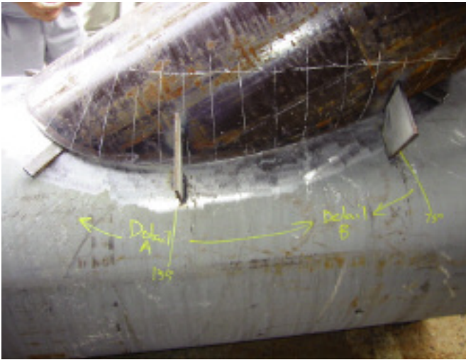
Fig. 4 — Measurement of the as-fit-up joint has begun. Note that the boundaries of the various Details have been marked on the chord member.
