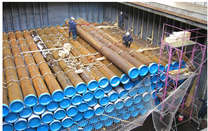
FIGURE 10. An order of longitudinally welded clad pipe being prepared for transportation.
