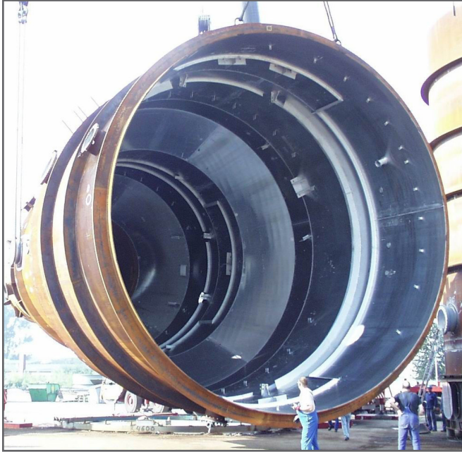
FIGURE 1. Partially completed vessels made from roll-bonded clad plate.
