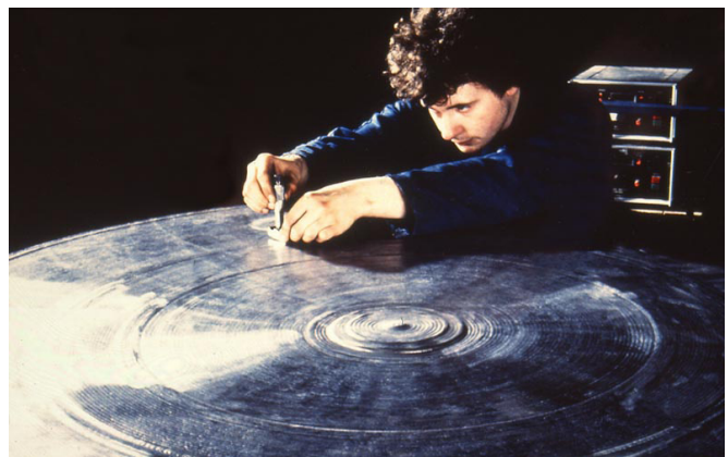
FIGURE 7. Heat exchanger tubeplate with 25mm thick weld overlay of Alloy C276.
