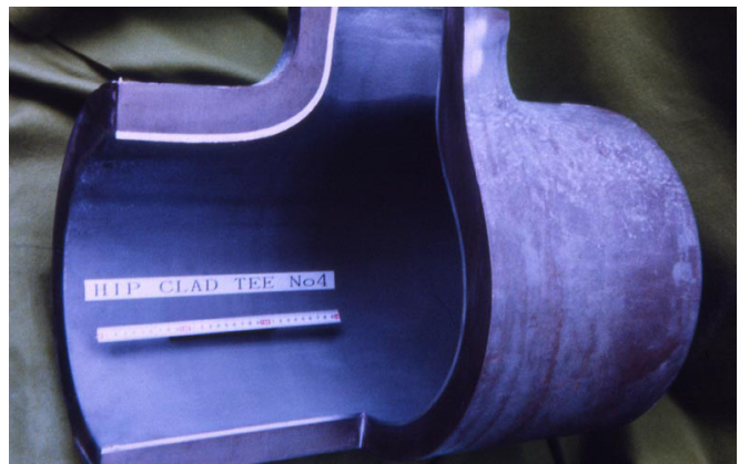
FIGURE 18. X60 Tee piece (16” x 8”) HIP clad with a solid lining of Alloy 825.
