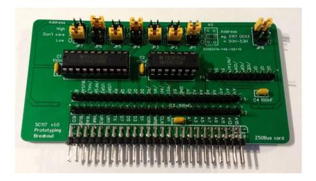
The card includes address decoding adequate for most I/O devices, thus saving the need to build a decoding circuit for every prototype. Address decoding is very flexible, allowing a configurable start address and a configurable range size.
