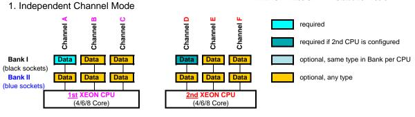
Independent Channel Mode allows all channels to be populated in any order Can run with differently rated DIMMs and use the settings of the slowest DIMM installed in the system
