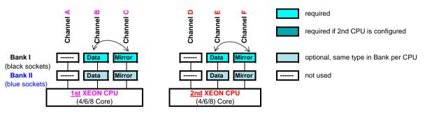
Mirrored Channel Mode requires identical modules on channel B / C (1st CPU) or channel E / F (2nd CPU) 50% of the capacity is used for the mirror => the available memory for applications is only half of the installed memory If this mode is used, a multiple of 2 identical modules has to be ordered.
