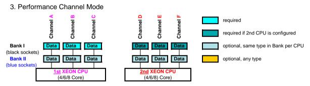
Performance Channel Mode requires identical modules on all channels of each Bank per CPU. If this mode is used, a multiple of 3 identical modules has to be ordered.
