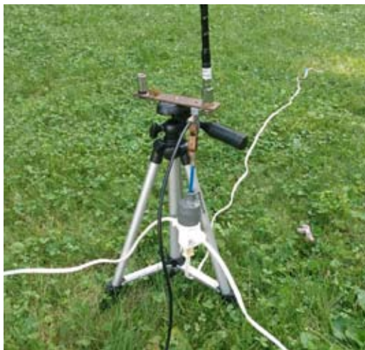
Radial Kit Deployed with hamstick antenna and tripod mount
