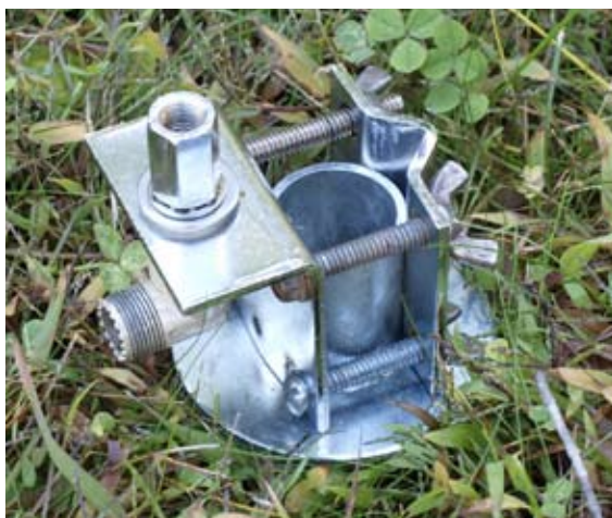
Pedestal in Ground ready to attach antenna and radials
