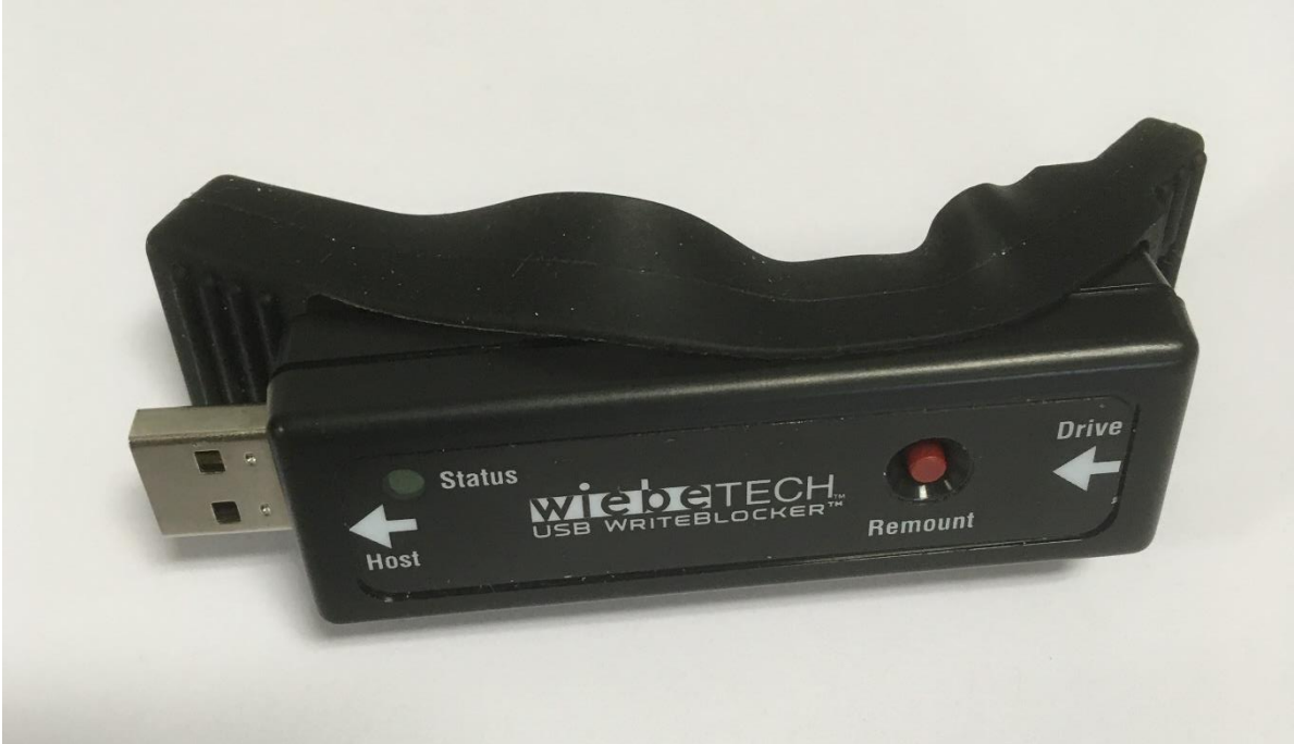
USB Writeblocker. Inserted between the PC and a disk drive it will prevent the PC inadvertently altering the contents of the disk.
