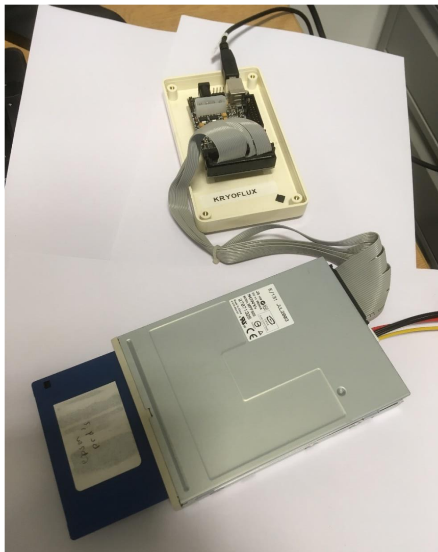
3 1/2" floppy disk in a disk drive connected to Kryoflux. The disk drive is powered from the mains, the Kryoflux is attached to a PC.
