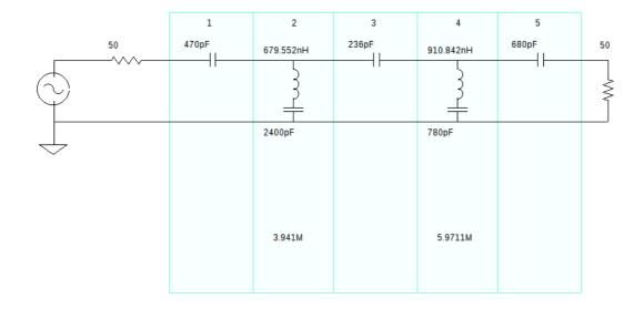
Design data: Bandwidth: 10M Family: Manual entry Q values: Inductors: 150 Capacitors: 1000 Maximum / minimum ratios: Capacitors: 10.169 Inductors: 1.3404 -Unbalanced preview
