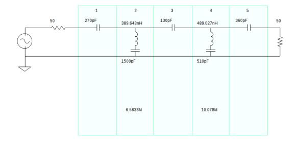
Design data: Bandwidth: 18.06M Family: Manual entry Q values: Inductors: 140 Capacitors: 1000 Maximum / minimum ratios: Capacitors: 11.538 Inductors: 1.2551
