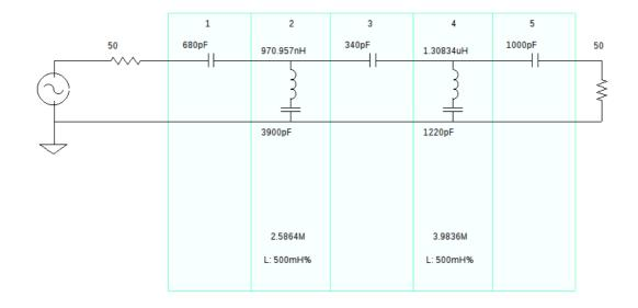
Design data: Bandwidth: 6.9M Family: Manual entry Q values: Inductors: 140 Capacitors: 1000 Maximum / minimum ratios: Capacitors: 11.471 Inductors: 1.3475 Unbalanced preview—
