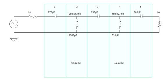
Design data: Bandwidth: 18.06M Family: Manual entry Q values: Inductors: 140 Capacitors: 1000 Maximum / minimum ratios: Capacitors: 11.538 Inductors: 1.2551 Unbalanced preview-
