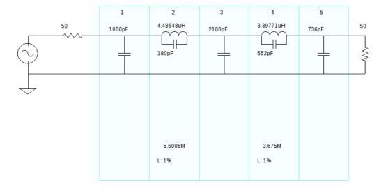
Design data: Bandwidth: 2.04M Family: Manual entry Q values: Inductors: 120 Capacitors: 1000 Maximum / minimum ratios: Capacitors: 11.667 Inductors: 1.3204 -Unbalanced preview-Normal - unbalanced Balanced - A Balanced - B 80 Metre Plot and schematic follow
