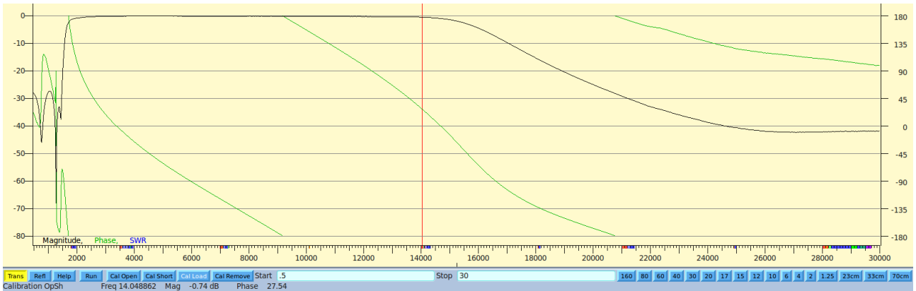
1.7 MHz HP Filter cascaded with a 14 MHz Low Pass filter in transmission mode
