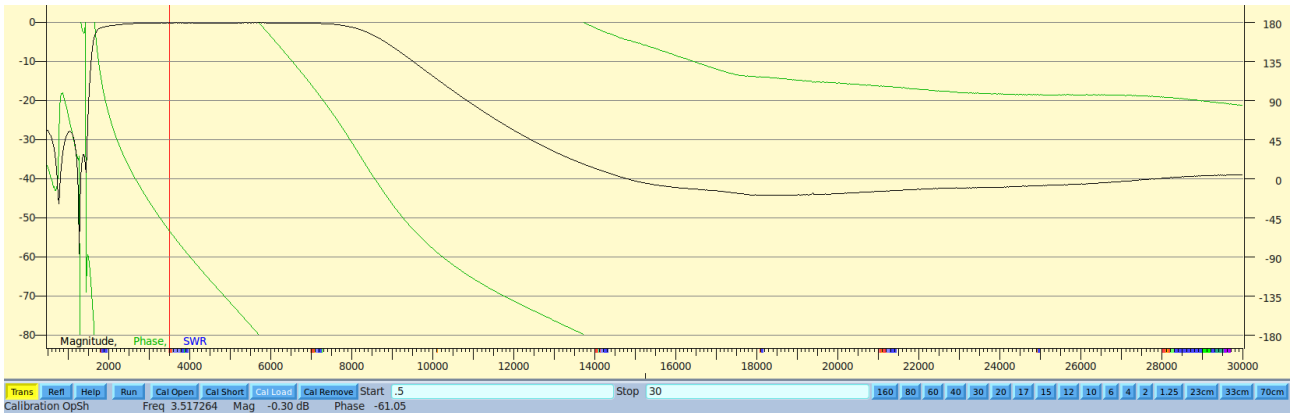
1.7 MHz HP Filter cascaded with a 7 MHz Low Pass filter in transmission mode
