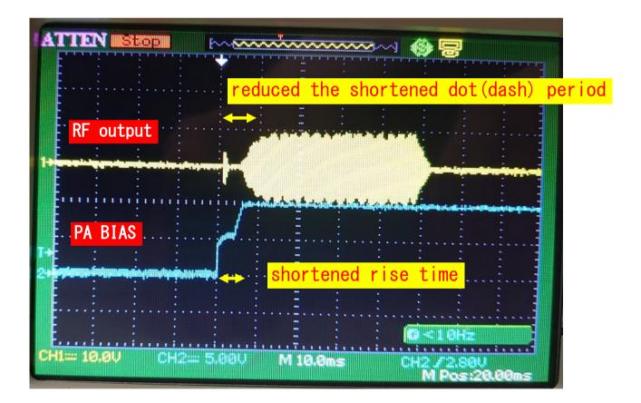
After replacement, if Key Down Delay is set to 10ms or more, the waveform is perfect !
