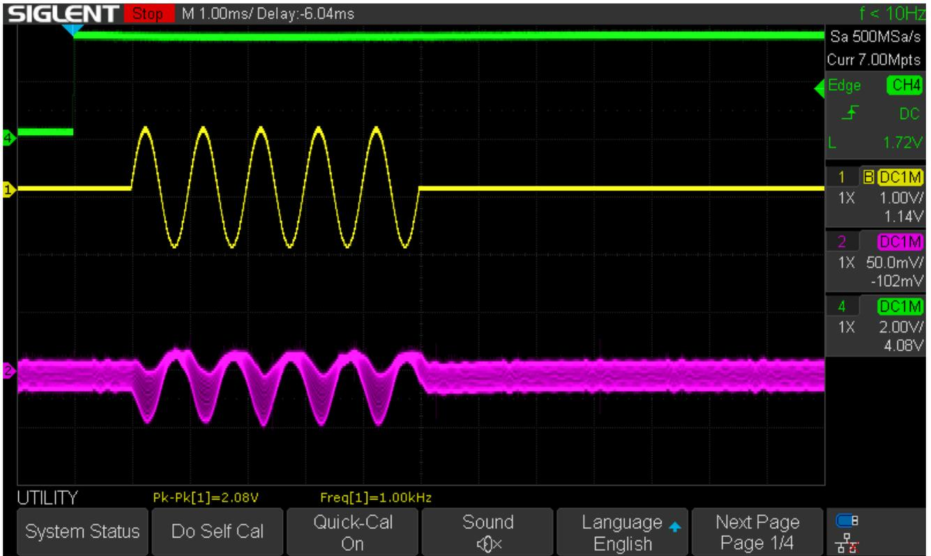
Noteworthy is that there is a 180 degree phase shift of the modulated signal, but essentially zero phase shift (or 0 time delay). Being the mixer frequency output is (A-B) the phase inversion makes sense.
