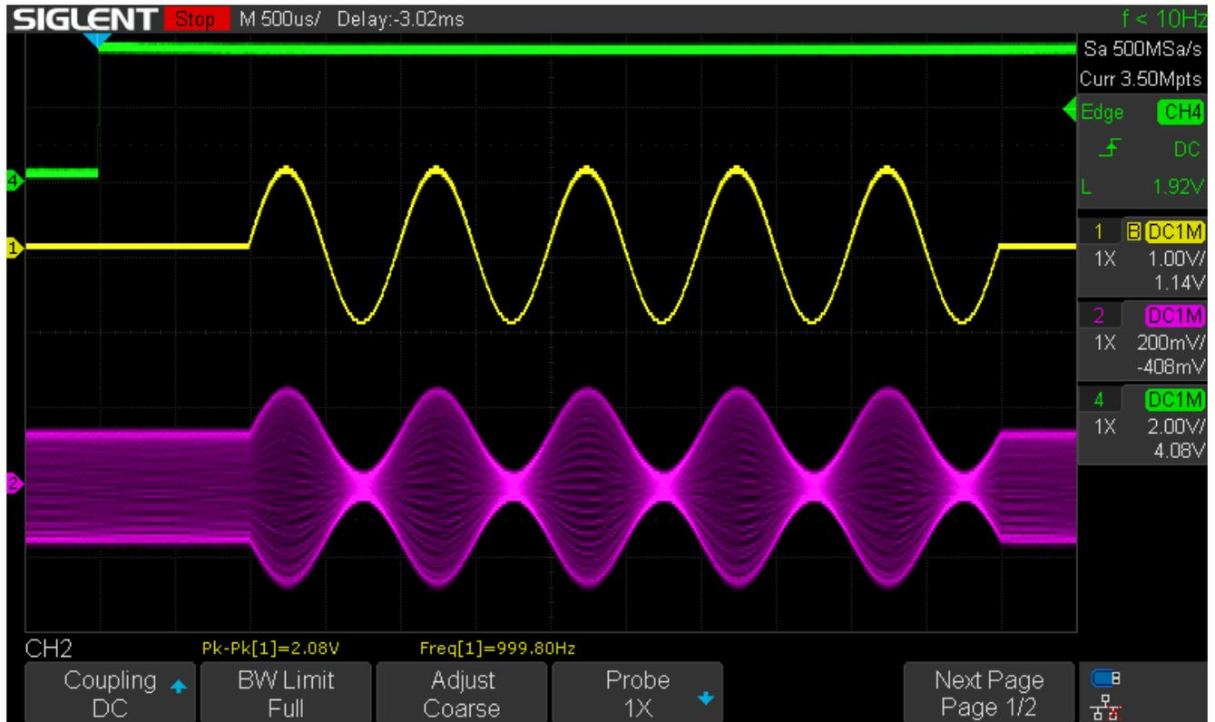
As seen from the scope capture, there is essentially no delay incurred (for purposes of this testing) by the generation of the test input signal to the RUT.
