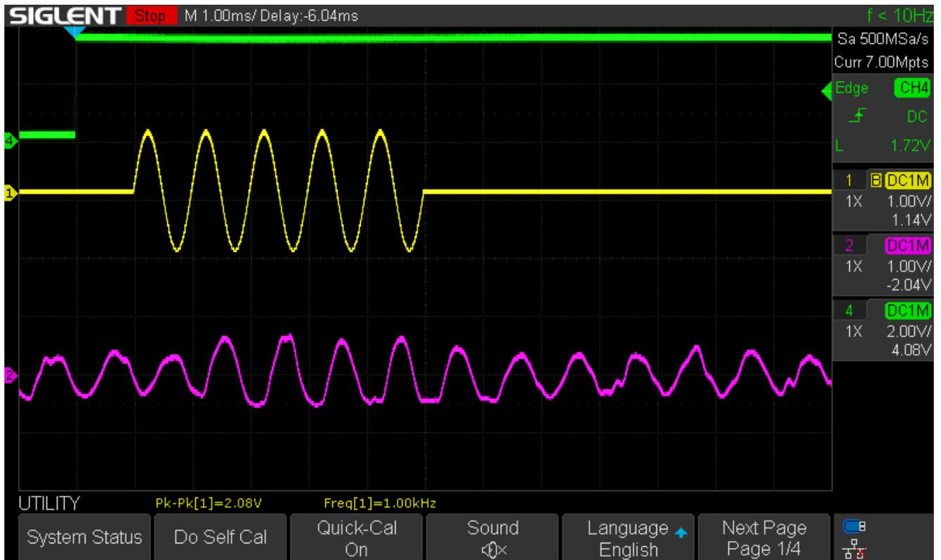
Harder to detect beginning of waveform, but the first higher amplitude waveform is the start of the burst.
