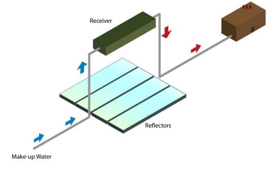
Several industrial processes require the transfer of heat, for which steam or other thermic fluids are used. Typically, these are heated using fossil fuel boilers or grid electricity. ARKA offers a novel and cost-effective alternative based on the bountiful energy of the sun. Using concentrated solar thermal power, our Industrial Steam Process equipment can generate enough energy to heat up the steam or thermic fluid to the required temperatures.
