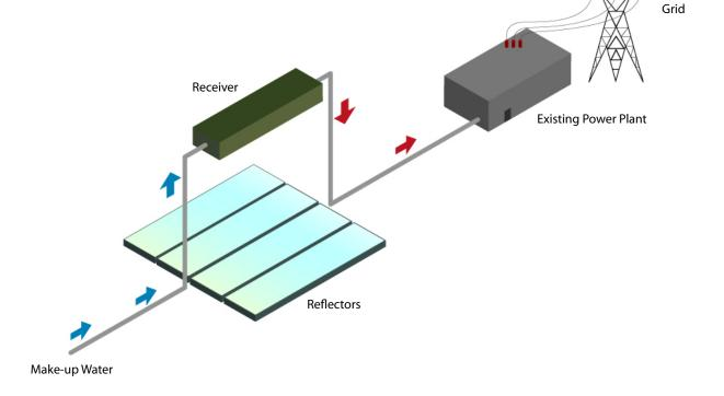
Existing coal or gas based thermal power plants can be further boosted with ARKA's Steam Augmentation systems. Delivering more steam to the turbines, these solar powered solutions are a cost-effective approach to increasing the output of the plant while also reducing the carbon emissions. Moreover, such steam augmentation increases the longevity of the plant.
