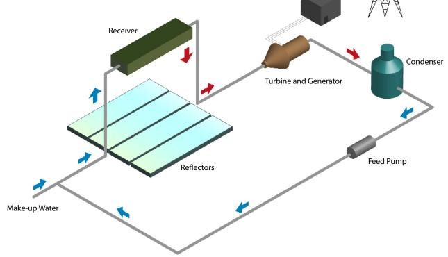
ARKA's Scalable Solar Power Plant uses indigenously designed technology to achieve unprecedented cost efficiency and embedded grid compatibility.
