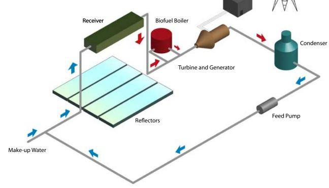
ARKA's Hybrid Solar Plant is a unique product that combines complementary energy sources to produce round-the-clock energy. Solar thermal power is used during daylight hours and an alternate source such as bio-fuel fills in for low-light and night hours. This translates into higher revenues and profits for our clients.
