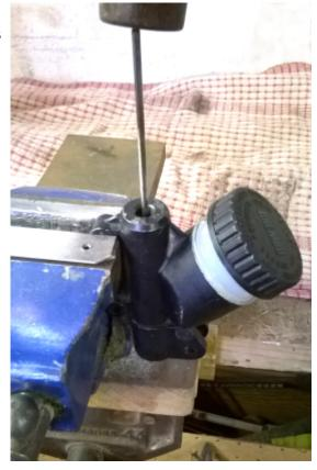
The internal parts came out of my cylinder in the order shown. The bore of the cylinder appeared in perfect condition, so the new parts were very lightly greased, with the supplied grease and reinserted in the same order.
