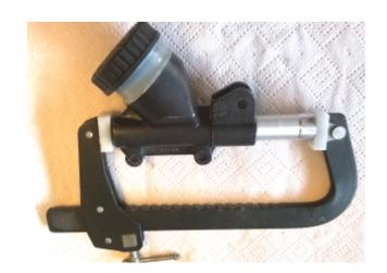
The T piece was then refitted with Locktite 542 and the lever lubricated and locked in place with the pin and circlips.
