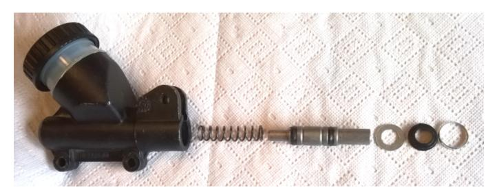
A tool is required to push the retaining collar into its groove in the cylinder body. A piece of aluminium tube was turned to 18.4mm OD and 40 mm long and a plug was also turned to fit the end of the tube. The whole assemble was then pushed back together with a cramp until the collar dropped into its groove.
