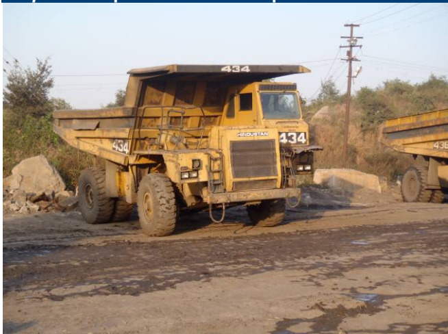
Dipka: dumpers used to transport overburden
